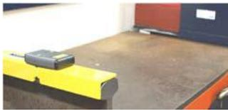
Place Lase-Align on rail, aligning the notch with the mark on the rail head and switch on the laser pointing towards the wall.
